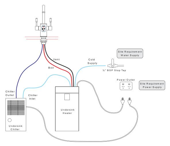
**WARNING**: The silicone piping from the Boiler/Chiller/Ambient tap to the Supatap must have a continuous fall to prevent the pipes from trapping water, twisting or folding. Failure to comply with this warning will cause the appliance to malfunction and void
