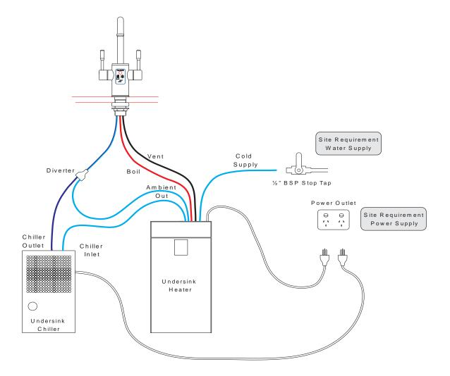
**WARNING**: The silicone piping from the Boiler/Chiller/Ambient tap to the Supatap must have a continuous fall to prevent the pipes from trapping water, twisting or folding. Failure to comply with this warning will cause the appliance to malfunction and void warranty. You may need to cut the silicone piping to achieve the length required for a continuous fall.
