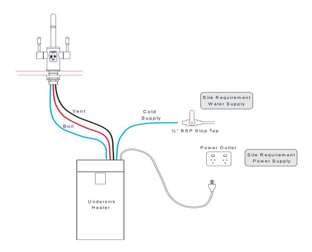
**WARNING**: The silicone piping from the Boiler/Chiller/Ambient tap to the appliance must have a continuous fall to prevent the pipes from trapping water, twisting, or folding. Failure to comply with this warning will cause the appliance to malfunction and void warranty. You may need to cut the silicone piping to achieve the length required for a continuous fall.
